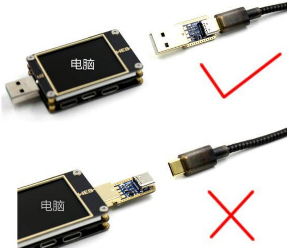
Note: Connecting or unplugging the PD spoofing cable from the computer needs to be unplugged or plugged in together with the adapter board
