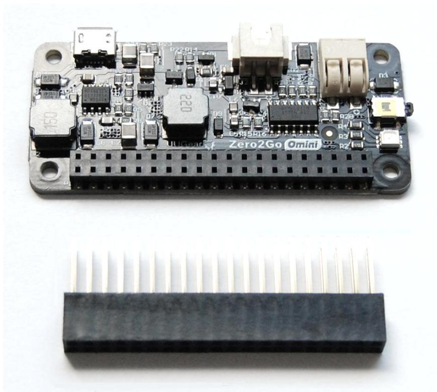
The 40 extra long pins on stacking header should reach the female header **via the holes on the back** of Zero2Go Omini. You can then place a steel ruler (or something
