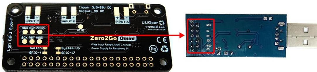
After doing so, you need to configure the programmer in your Arduino IDE. If you are using USBasp, just select menu “Tools->Programmer->USBasp (ATTinyCore)”. Now you can upload the firmware.
