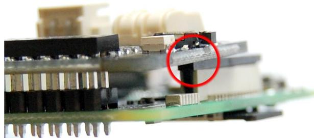
In order to make reliable connection, we suggest to use a [stacking pin header](#) (not included in the package).
