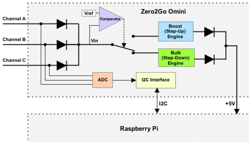
Three input channels (A, B and C) are merged as  $V_{in}$  with 3 schottky diodes. The comparator will compare  $V_{in}$  with an internal reference and decide whether to use step-up or step-down engine. When  $V_{in}$  is lower than 5.5V, the step-up engine will be used; When  $V_{in}$  is 5.5V or higher, the step-down engine will be used instead. The outputs of both engines are also merged with 2 schottky diodes.
