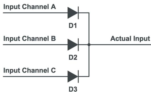
In Zero2Go Omini, these diodes (D1, D2 and D3) are high current schottky diodes. Thanks to them, the input channels are separated, and they all have reverse polarity protection.
