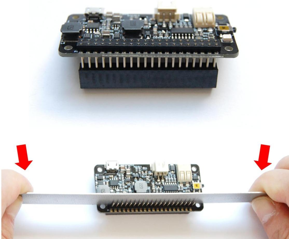
If you want to take off the stacking header from Zero2Go Omini, the proper way is to put your Zero2Go Omini upside down, and let the 40 pins contact a flat surface (e.g. the desktop), hold the two edges and press the board down. That way the stacking header will be taken off safely. See the figure below:
