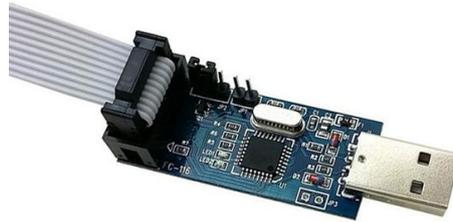
The USB programmer can communicate with Zero2Go Omini board via Serial Peripheral Interface (SPI). You will need to wire the pads (pins) with same name together:
