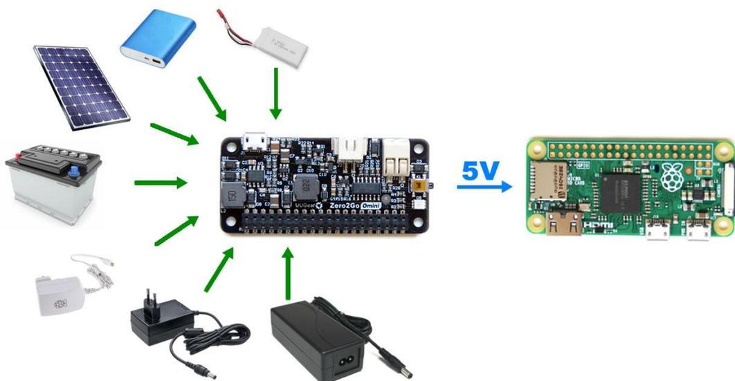
The board size of Zero2Go is exactly the same with Raspberry Pi Zero (W), and can be mounted on Raspberry Pi Zero or other Raspberry Pi models that have 40-pin header.
