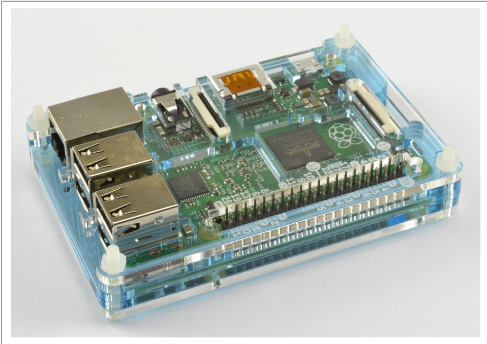
Figure 1-2. A Raspberry Pi 2 in a PiBow Coupé
