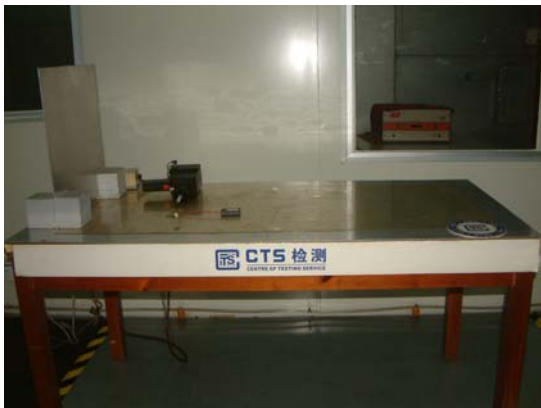
7.2. Photo of electrostatic discharge Immunity measurement (E.S.D.)
