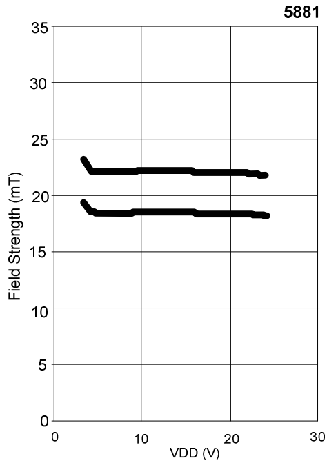
11.1 Typical Magnetic Switch Points vs V_{DD}
