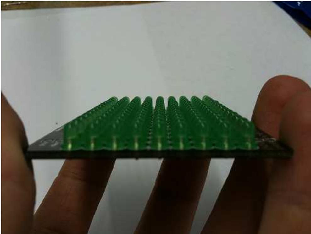
By looking down the rows and columns, you can see which LEDs are straight or crooked. This is much easier to fix when only one lead is soldered in, and it's easiest to find them along the way. Straightening them all at the end is quite a bit more difficult.
