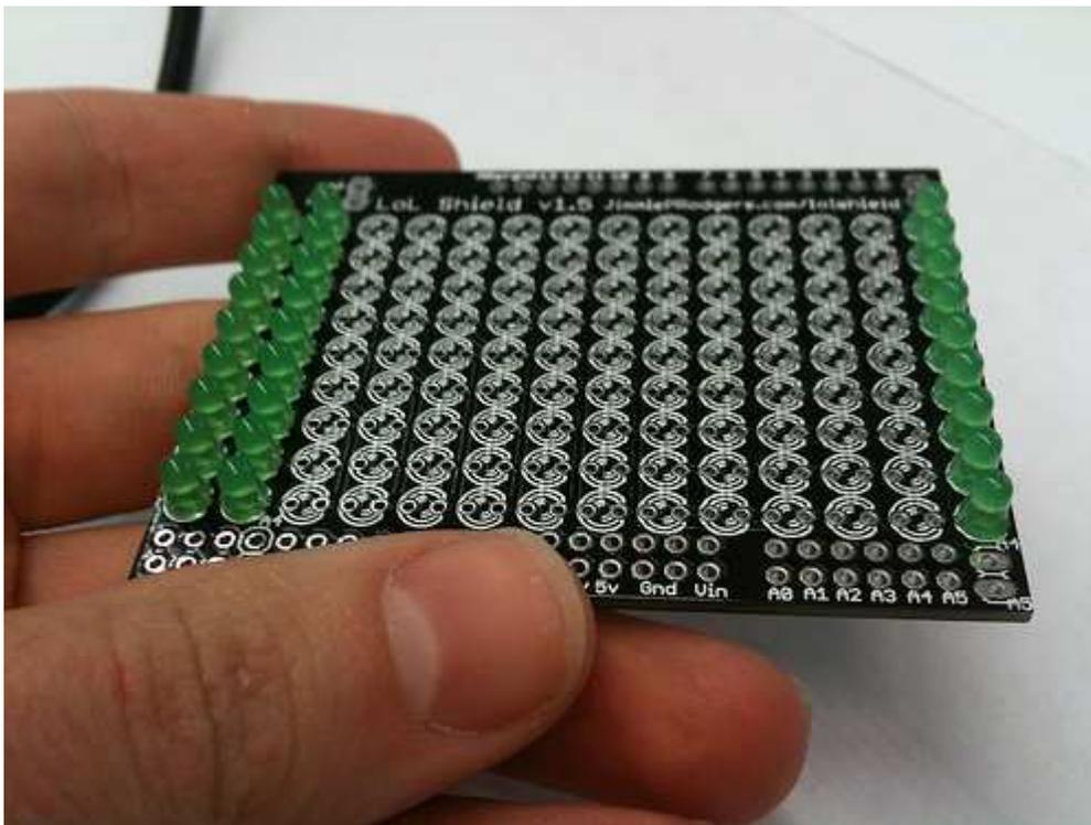
To straighten the LEDs you solder one lead of each LED so that it sticks to the PCB. Then you gently place your finger on the LED and press on it as you re-heat the soldered joint. By pressing it flat against the PCB, the LED will automatically straighten up. Keep filling in each column and work your way down in this way. Some people also find it
