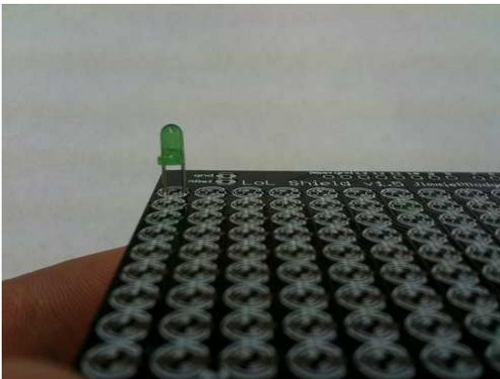
If you look at the silkscreen (the white markings) on the PCB (printed circuit board), you will find that a little notch has been taken out of the LED drawing as well. You are going to be placing all of the LEDs in the same way, matching both the notch and short lead to the marked spot on the PCB. Essentially, with the text being upright and readable, you
