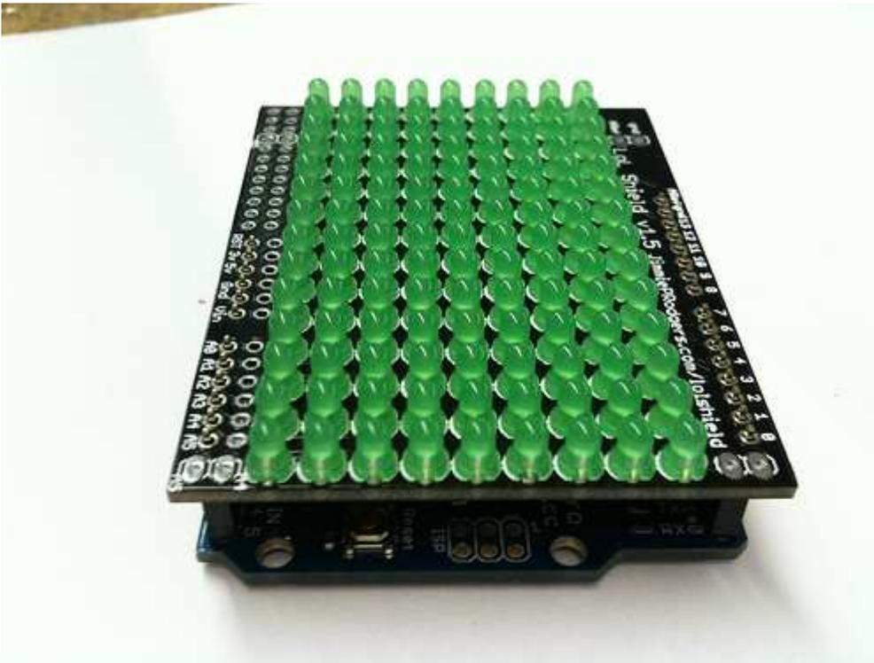
Simply place the LoL Shield on top of the headers and solder them in place. Trying to line up headers so that they stick comfortably in the Arduino is very hard. This keeps them nice and straight. You don't have to worry about damaging anything. Just heat it long enough to solder it in place, and it should work out fine.
