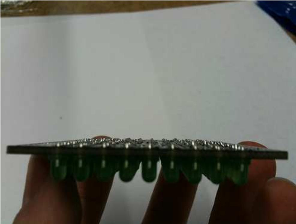
Once all of the LEDs are straight, you should try and clip the leads as short as you can without lifting pads off the PCB. Clip just at the top of the solder blob (it's okay to cut a bit into it). This is mostly important around the area above the USB port.
