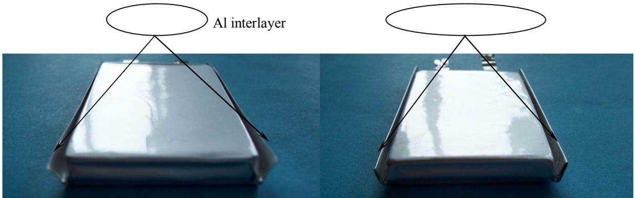
Fig.2. Single folding edge schematic of PL cells
