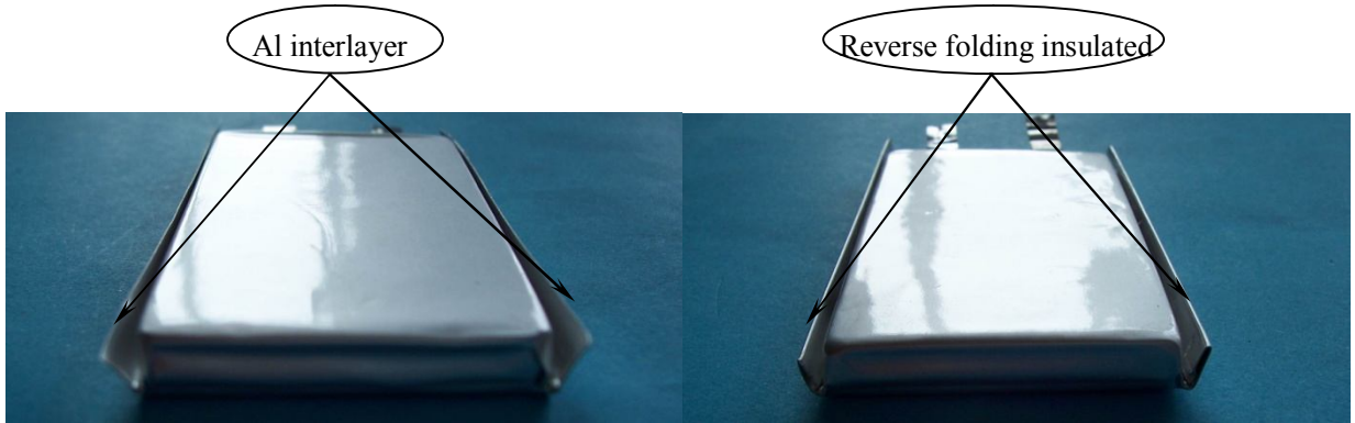
Fig.2. Single folding edge schematic of PL cells schematic of PL cells
